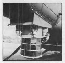
AN/ALQ 144 infrared jammer was fitted to army aviation helos flying in direct support of MilGroup operations in El Salvador. Such equipment came in response to the January 1991 shoot-down of an American Huey by FMLN small-arms fire. Other improvements included Kevlar floor mats and engine armor.
